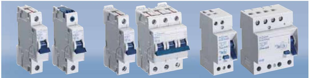
**Miniature circuit breakers,** 1-pole, 2-pole and 3-pole, as well as 1+N and 3+N 0.3 to 63 A, tripping characteristics B, C, D, K, Z Miniature circuit breakers, UL508 and CSA approved
